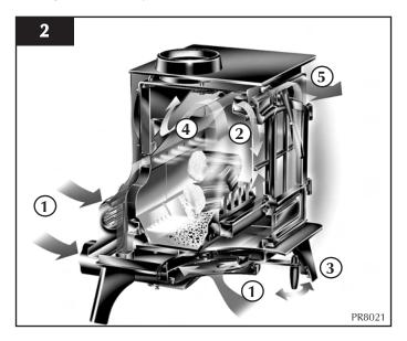
1) Primary Air - burns the fuel under the fuel bed. For use with solid fuel and initially with wood fires.
